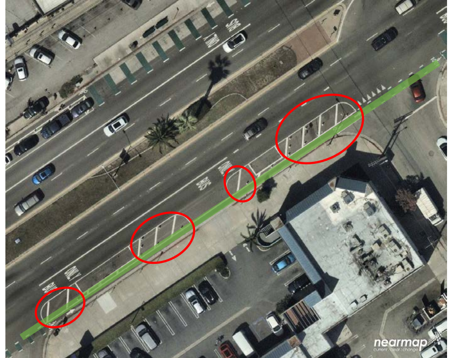
Example: Parking-protected bike lane with no parking immediately before and after driveways and intersections
